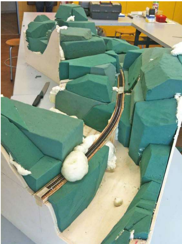
The polyurethane foam is ready to be trimmed away, before it fully hardens.
