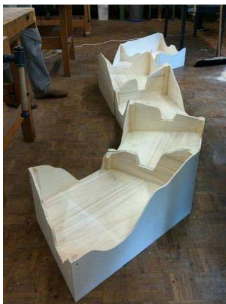
After the first working session, the completed woodworking gives an idea, what the Abo Canyon section is going to look like. The fascia is already cut to shape.
